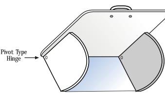
Door is hinged with an attached security panel to prevent removal of donations.
